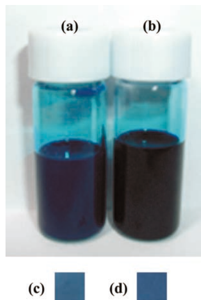
Fig. 8 a Colored latex containing phthalocyanine dyes (B7). b THF solution of phthalocyanine dyes. The dye contents of a and b are equal. c and d show the color of a and b spread on paper
